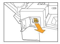
Press the areas indicated by the arrow ① to release the hooks, and remove the staple case.
