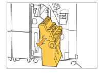
Remove the staple cartridge by lifting it up after slightly lifting it down while holding the cartridge handle.
