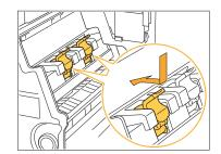
Align the  ${\color{red}\blacktriangle}$  marks on the cartridge and booklet unit when attaching the cartridge.
