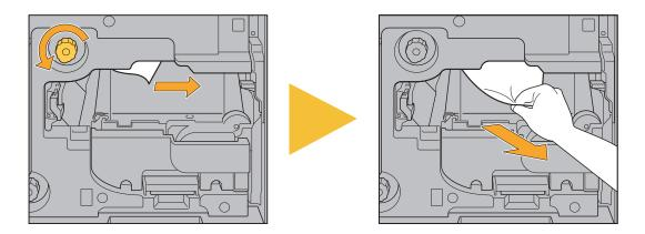
• If a paper jam occurs when printing multiple sheets of paper, the sheet of paper that caused the paper jam as well as other sheets of paper may remain in the transfer path. When using an internal dial to remove jammed paper, turn the dial four or five times after removing the first sheet of paper, to check for other sheets of paper.
