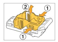
4 Insert the front part of the new staple case into the cartridge, and then insert the back part.
