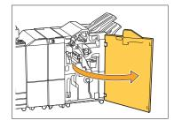
2 Release the lock by moving the lock lever to the unlock icon (open) position on the left.
