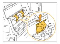
4 Open the staple cartridge cover and remove the jammed staple.
