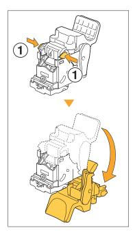
6 Press the areas indicated by the arrow ① to release the hooks, and remove the staple case.
