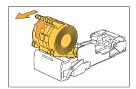
Insert a new staple case into the staple cartridge.
