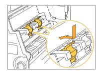
Be sure to install the staple cartridge to the position aligned with the  $\, \blacktriangle \,$  mark of the booklet unit.
