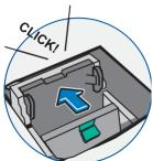
9. Replace the ink tank cartridge. Follow steps 5 - 10 in *Replacing the Ink Tank Cartridge* in this chapter for more information.
