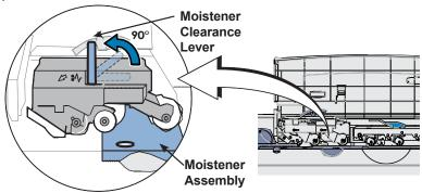
3. If necessary to gain access to the material, push down on the blue button and slide the moistener assembly out of the deck.
