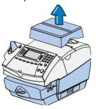
2. Open the ink access cover. At the screen with the red X, select "Replace Ink Tank". A "Moving Ink Tank" message displays.
