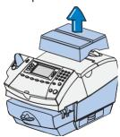
2. Open the ink access cover. At the screen with the red X, select "Replace Print Head". A "Moving Ink Tank" message displays.
