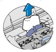
2. Pull the moistener *tank* (located under moistener bottle) straight out towards you. Gently lift the tank up and out.
