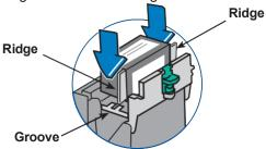
7 Rotate guard back to closed position and be sure it latches. Press on the two half-circle shaped pads on either side of the green latch until the latch snaps into place
