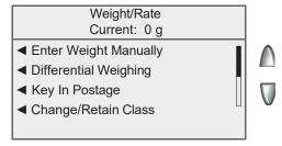
5. At the "Start Differential Weighing" screen, place the items on the scale.
