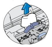
3. Unscrew the moistener bottle cap and fill the moistener bottle with Pitney Bowes E-Z Seal® sealing solution. We recommend E-Z Seal® because it helps keep your moistener clean and improves sealing efficiency.
