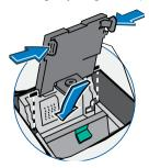
8. Push the print head back into place. You should hear a click when it is seated correctly.
