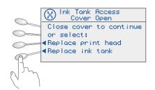
C. Open ink cartridge guard, remove ink cartridge, and close ink cartridge guard.
