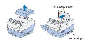
B. Select **Replace ink tank** to move the ink cartridge carriage to the replacement position.
