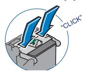
14. Close the cover. The system automatically recognizes the new cartridge and in a few moments returns you to the Home screen.
