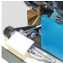
Then the Pick Arm begins to rotate 180 degrees and prepares to accurately place the product
