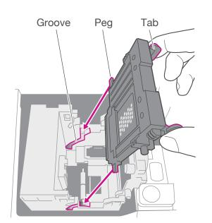
3d. Squeeze the tabs and slide the printhead pegs into the lower set of **grooves**.
