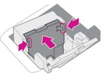
3e. Keep squeezing the tabs and push the printhead flush against the wall. Tabs will snap outward when placed correctly.
