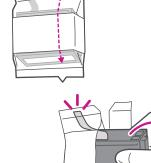
3f. Unwrap the ink cartridge and make sure you remove the silver foil strip from the ink cartridge.
