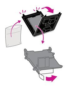
3c. Unwrap the printhead and remove the protective strip.
