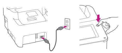
4a. Connect SendPro C to a power source and turn on the power switch.
