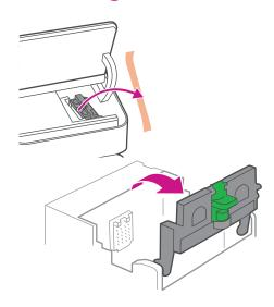
3b. Remove the packing tape from the ink carriage, and open the guard.
