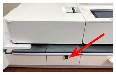
2. Open the feeder access cover to access the moistener bottle.
