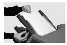
2. Aerate (fan) the stack of paper to ensure that individual sheets are not stuck together.
