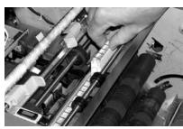
Push down on the blue tab to return the upper felt assembly to its operating position. Make sure that the blue latches (A) spring out and fully latch into position.
