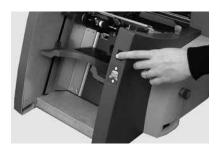
Use the side guide adjustment knob to adjust the side guides to the width of the envelopes. Once adjusted, back-off the adjustment knob 1/4 turn.
