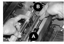
4. Push the latch (A) back, grasp the upper sealer felt (B), and slide it towards the front of the inserter
