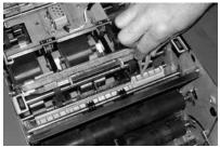
Install the four new felts into the sealer tank. They will only fit one way. Push them fully down into the tank.
