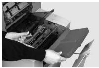
Squeeze both blue tabs (A) together and lift one tab (B) to gain access to the sealer unit felts.
