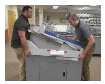
Then slowly lower until the bottom of the top piece is flat against the top of the base assembly.
