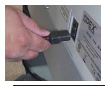
Plug in the main power cord into the rear of the machine and power on to configure.
