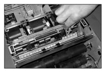
Install the four new felts into the sealer tank. They will only fit one way. Make sure to push them fully down into the tank.
