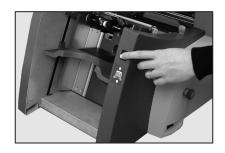
Adjust the side guides to the width of the envelopes. Use the side guide adjustment knob, then back-off 1/4 turn.
