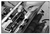
Push down on the blue tab to return the upper felt assembly to its operating position. Make sure that the blue latches (A) spring out and fully latch into position.
