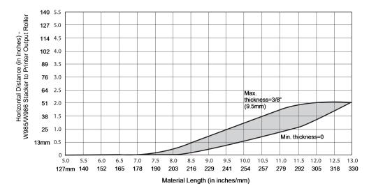
The top chart is used to determine the distance to set between the stacker deck and the printer output roller. This is done by adjusting the height of the stand.
