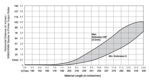
The top chart is used to determine the distance to set between the stacker deck and the printer output roller. This is done by adjusting the height of the stand.
