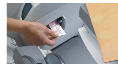
Step 2 – Feed envelopes through the DM1000™ or press the tape button for parcels. The correct postage is then imprinted, and the piece is ready to go.
