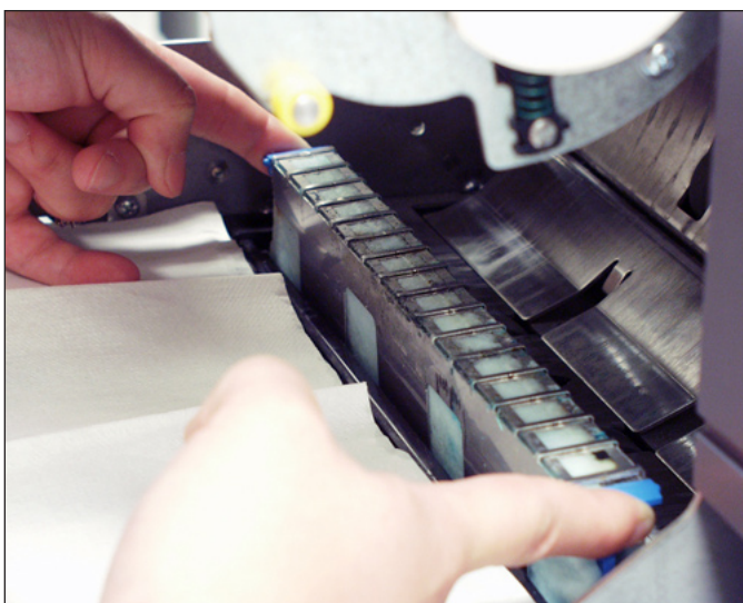
Figure 5.3: Removing the Old Wick Cartridge
