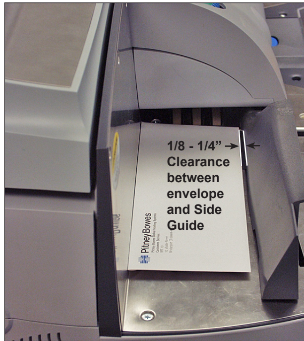
Figure 7.16: Clearance Between Envelope and Side Guide
