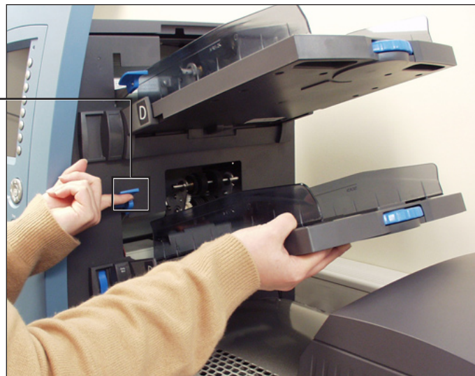
Figure 3.1.1: Lift the Separator and slide the Tray into the tray mounts.
