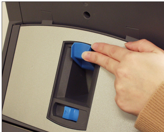
Figure 3.8.1: Push up on the Separator Gap Lever
